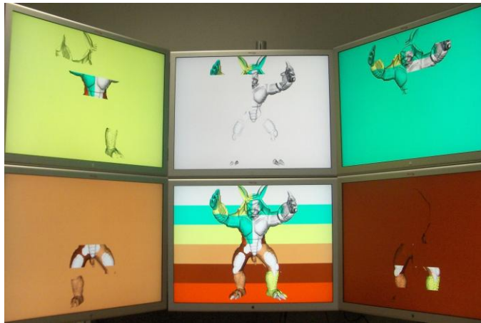
Figure 5 - A six pipe sort-last, direct-send configuration using Equalizer(Equalizer)
