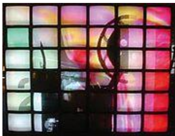
Figure 3 shows an example use of sort-first rendering on a video wall. Each computer in the video wall renders a portion of the viewing volume, and the final image is the summation of the images on the monitors that make up the video wall.
